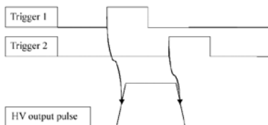
Fig. 3. Control timing charts for two-pulses controlled drivers
