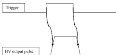
Fig. 4. Control timing charts for single pulse controlled drivers
